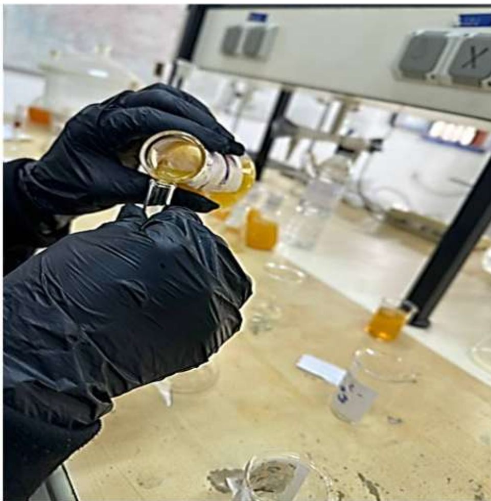
Figure 3. Addition of ferric reagent during color development.
